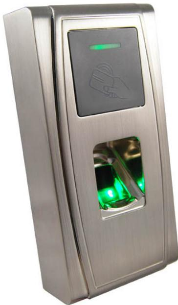
The **FingerPass EX** is a biometric terminal intended for time management and physical access control. The terminal allows recording the arrival and departure events of the company's employees and managing electromechanical and electromagnetic door-locks, turnstiles, gateways opening them upon successful verification of users by their fingerprints enrolled earlier into the system.
